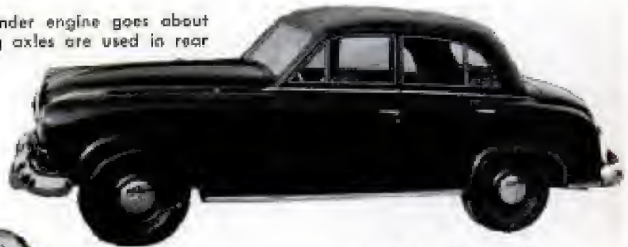
RILEY Pathfinder, below, seats six, has four cylinders, two camshafts, hemispherical combustion chambers, a torsion-bar front-suspension system
